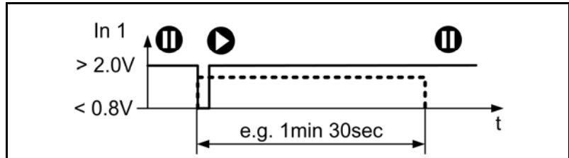
Fig. 64: Start ml/min with time counter pulse control
