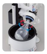
Implementation of automatic reverse revolution to be suited for drying-out and concentration of powder and solid substance etc.
